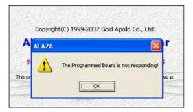
4. Please re-check the ALA26 programmer and printer port are well installed or not. If connection succeeds with the ALA26 programmer, the system enters the Main Menu.
